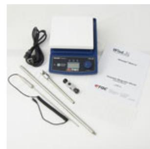
**Standard delivery** Digital hotplate magnetic stirrer, Power supply curt, operation manual, display scratch cover, clamp + sensor holder, PT100 temperature sensor, stand rod.
