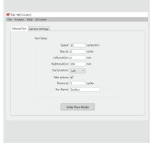
② Open Software and add the parameters on Manual Run. Press Enter. The device will run the defined Setup.
